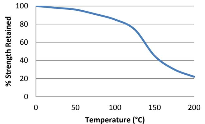
"Hot strength" shear strength tests performed on mild steel. Fully cured then conditioned to pull temperature for 30 minutes before testing.
