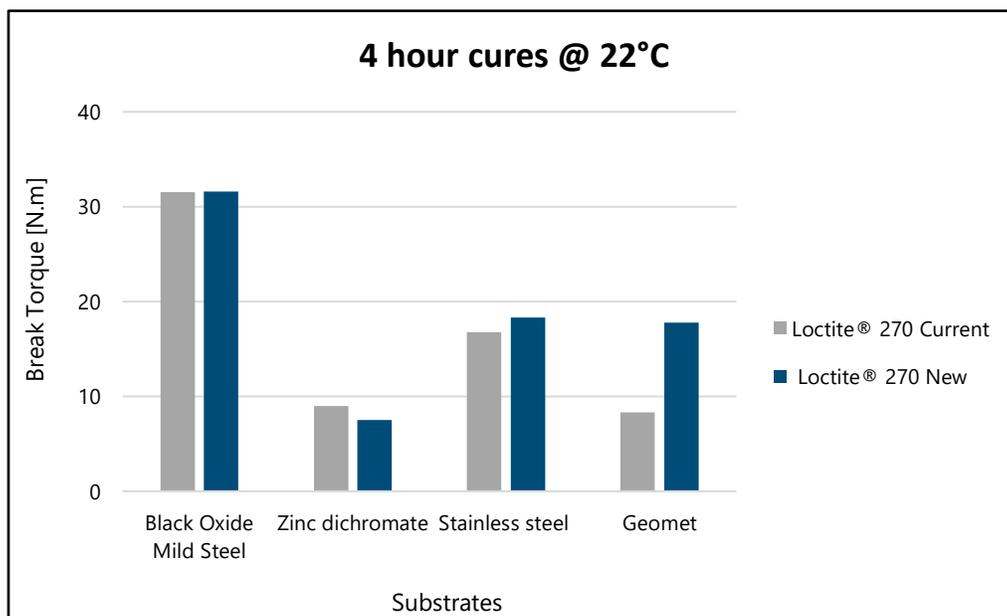
**Conclusion:** Consistent cure performance is observed for Loctite® 270 Current and Loctite® 270 New on all substrates tested.
